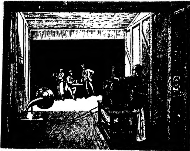
Projection room (about 1894), showing phonograph attached to kinoscope for synchronization of sound and picture. ( Century Magazine , 18, 207, 1894.)
